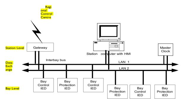
System Architecture of Substation Automation
